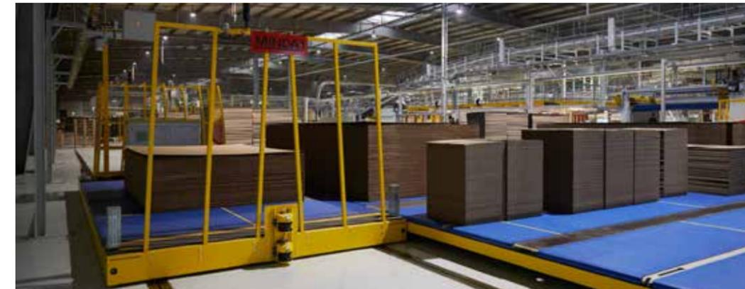
The MINDA conveyor system transports 1,100,000 m<sup>2</sup> of corrugated board per day
